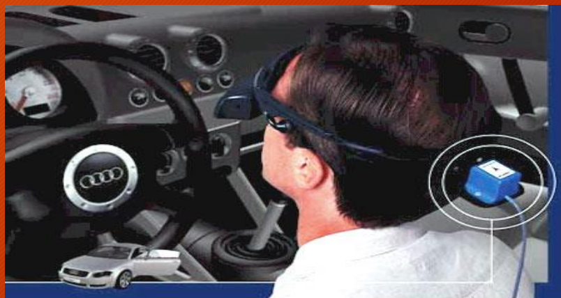
3D-BIRD mounted on Sony LDI-100 HMD. Audi TT Coupe virtual interior and exterior environment courtesy Eon Realty, Sweden.
